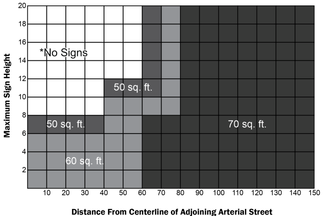
Figure 5.9.5-A: Freestanding Sign Adjacent to an Arterial Street
