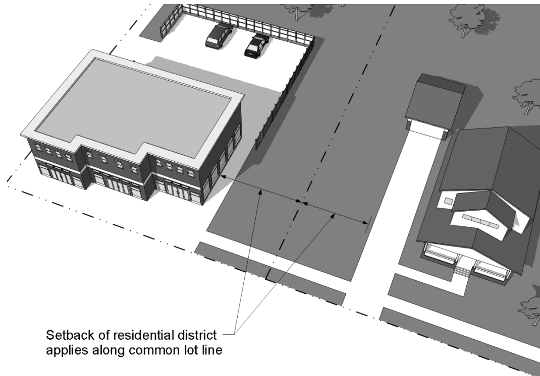
Figure 3.7.5-A: Transition of Side Yard Setbacks
